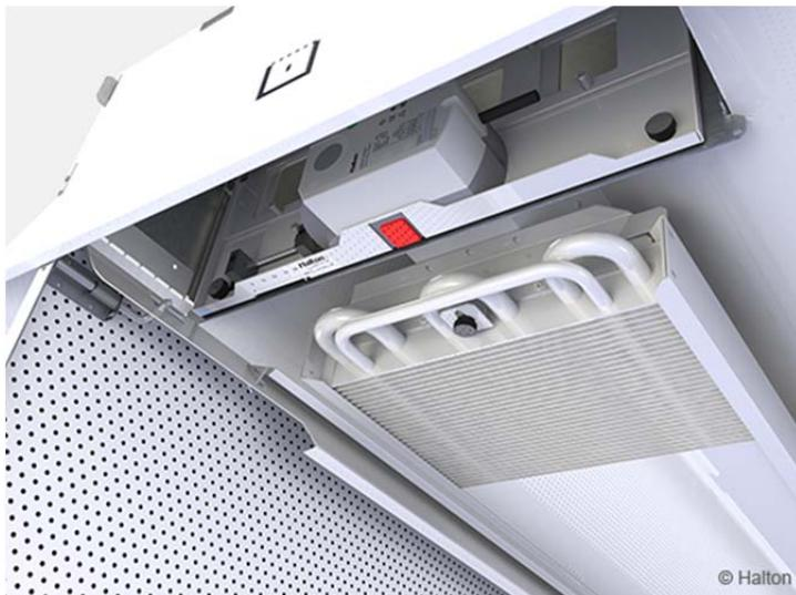
The Halton Air Quality (HAQ) control unit's position and the selection of chilled beam nozzle size allow adjustment of the primary air flow rate in the space. The separate air flow adjustment damper installed in the duct branch is used for balancing the air flows in the ductwork.
