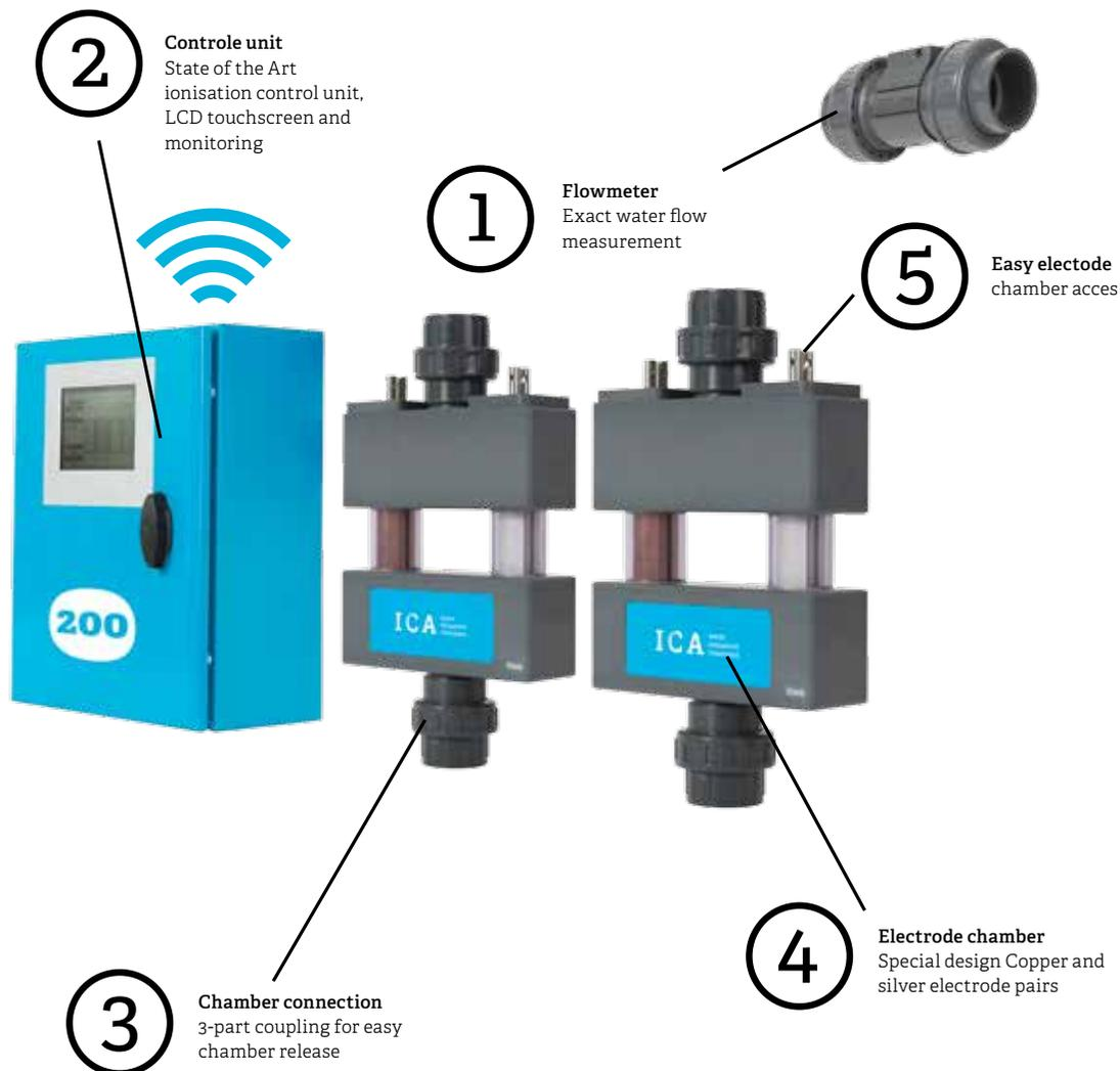
Our ICA Ionisation water treatment system successfully eliminates Legionella bacteria from water. It's a precision controlled process based on the ionisation of copper and silver. This state-of-the-art technique actually finds its origin in a method that's been used over hundreds of years to eliminate harmful bacteria in our drinking water. Today, we are the only Dutch supplier of ionisation systems included in ECHA's "Article 95" list as authorised suppliers for copper and silver.
