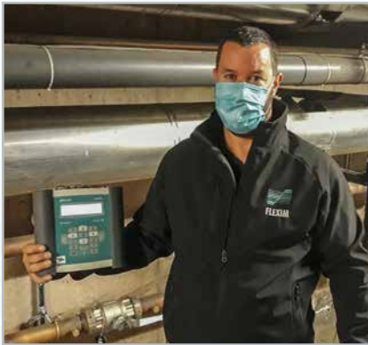
With his portable FLUXUS® G601 CA Energy, FLEXIM's service engineer was able to convincingly demonstrate on site the suitability of the non-invasive ultrasonic technology for the measuring task.
