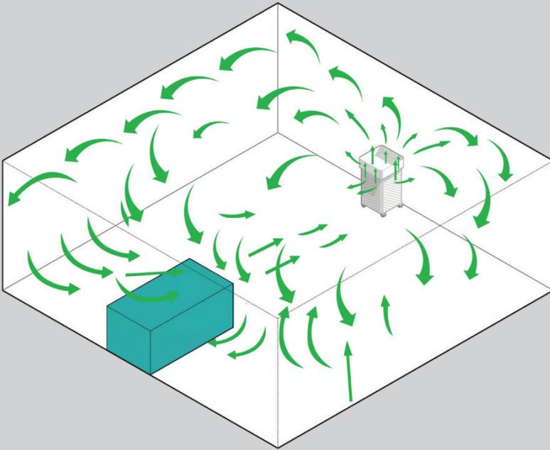
The flow from the Air Sentry® system forms a rotational motion within the slow moving air stream, throughout the entire room.
